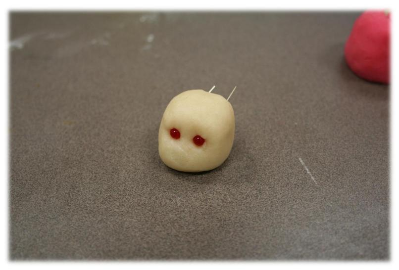
Cover the Head with Conductive Dough and Make Sure the Bottom LED's Make Contact with the "Skin". Cover the Other Motor Terminal and Top LED Leads with Another Section of Conductive Dough. Fill the Remaining Area with Insulating Dough and Cover with Conductive Dough.
